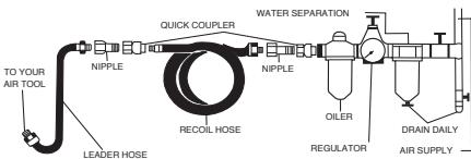
**WARNING:** Ensure that the air system is fully drained and the compressor is switched off, before connecting the filter regulator.
